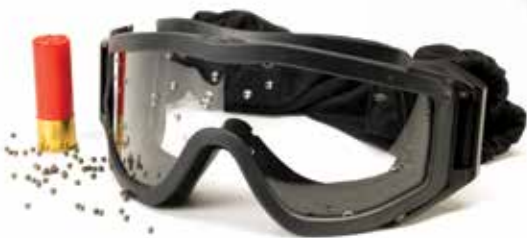
Loadout ballistic goggle shot with 12 gauge shotgun and 2 ¼ inch steel #6 at 25 yards.
